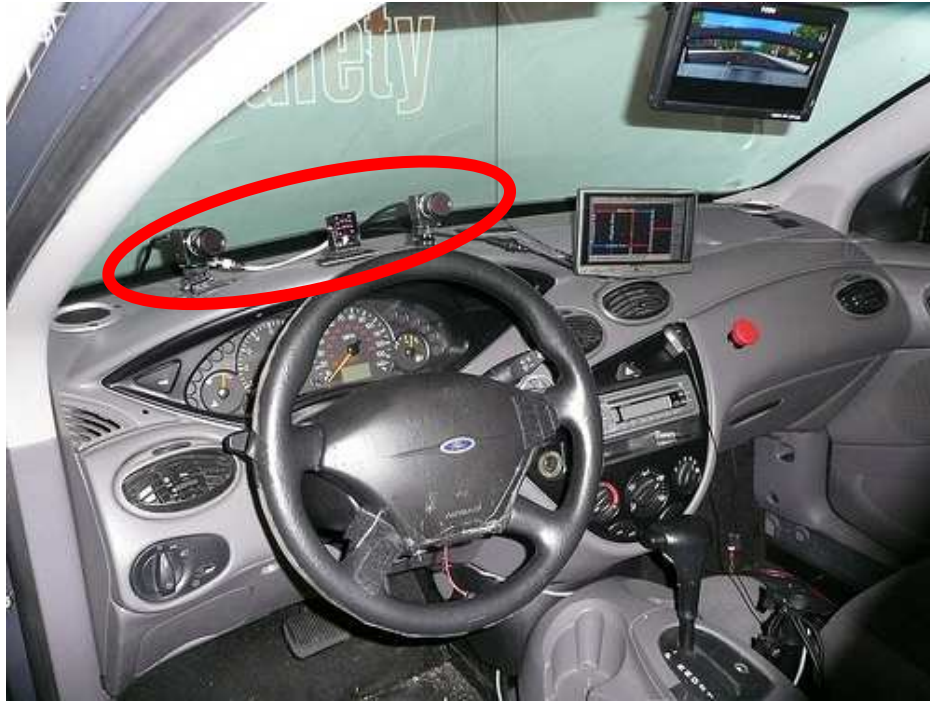
Figure 4.3 Eye-tracker cameras installed inside of the simulator cab.
